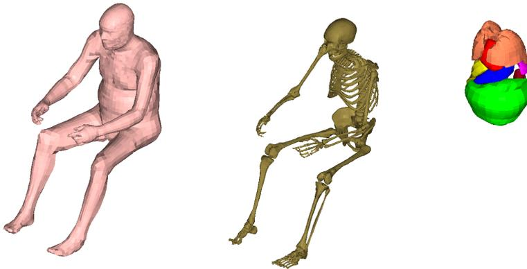
**Figure 2.** MADYMO Finite Element Occupant Model in automotive seating position.
