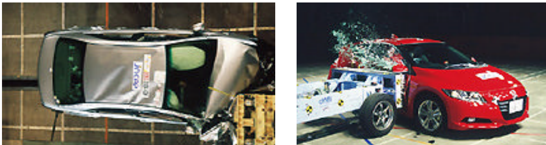
Figure 21 Examples of crash tests in JNCAP, Japanese NCAP – frontal partial overlap test (left), side impact test (right) [64]
