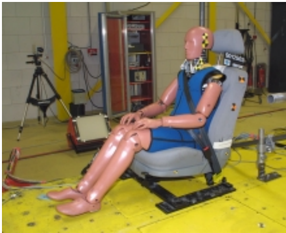
Figure 2: Overview of test set-up for RID 2 evaluation.
